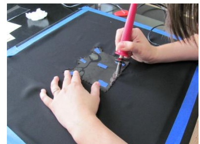
The Mylar tracing is taped to the polyester sheer and carefully cut using a commercial wood-burning tool.
