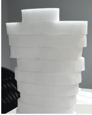
Cut disks stacked up before gluing and shaping
