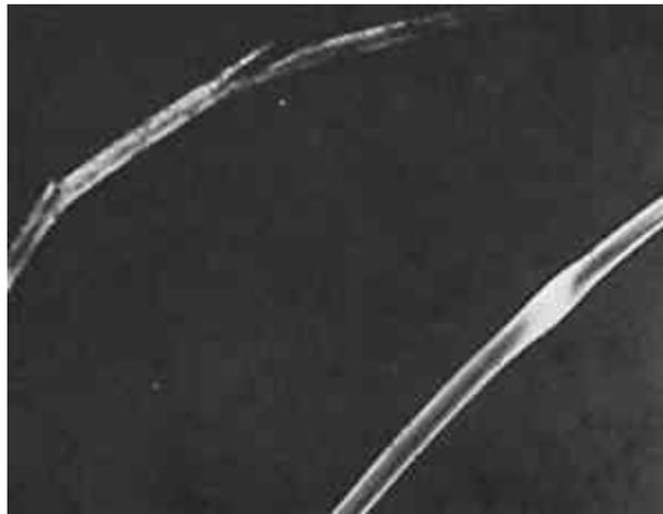
Fig. 2. Partial fractures in silk fiber, indicating brittleness. Green-stick fracture is characteristic of silk. Crossover indentation in lower fiber. 500x, 73° crossed polars.
